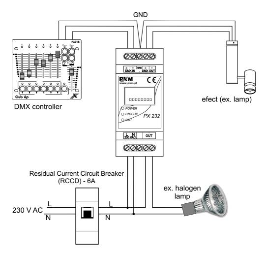
PX232 must be connected to the DMX line in series. This means that to the DMX IN terminal control cable should be connected, and then from the DMX OUT terminal the control cable should go to other DMX receivers.
