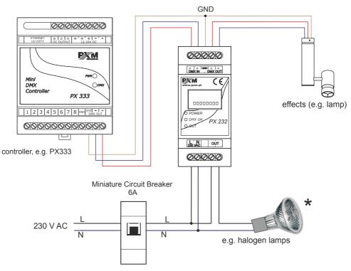
\* - in the case of inductive lead, additional power contactors should be used
