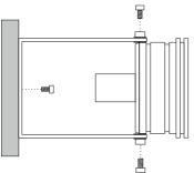
The lamp is attached to the holder with two M3 Allen screws and can be rotated vertically. The handle, on the other hand, is attached to the ground with an M5 screw, which in turn allows for rotation in the horizontal plane.
