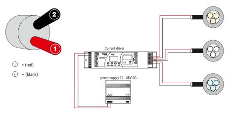
b) connecting a monochrome lamp to the power supply
