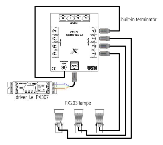
**NOTE!** The lamps should be connected starting from inputs 1, 2, 3, etc. If, for example, there are lights *only* on outputs 1, 2 and 3, it means that a built-in terminator (*terminator cable*) should be connected to output number 4. If all 12 outputs are used, then the built-in terminator (*terminator cable*) is not connected.
