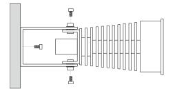
The lamp is attached to the holder with two M4 Allen screws and can be rotated vertically.
