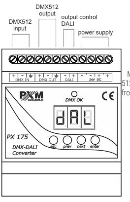
Module PX175 DMX/DALI Interface has DMX-512 input and DMX-512 output, and additional DALI output. The device is powered from 24V DC.
