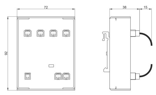
**NOTE!** Remember to leave at least 1.5 cm for cables connected to the device using plugs.
