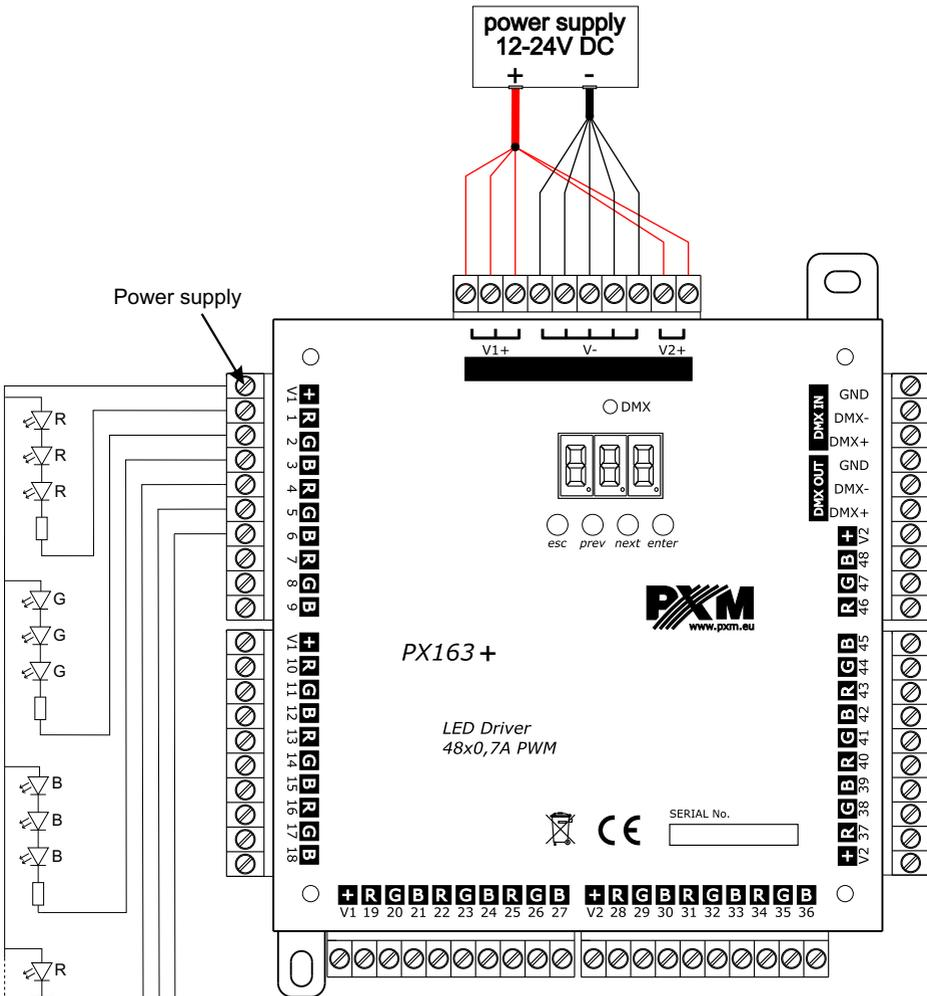
The receivers are connected to the driving and power supplying outputs as shown in the figure. The specified number of light sources can be on each line, depending on consumed power, and the load of each line is max. 700mA. Therefore, after connecting all the receivers, add all lines and select the adapter with adequate power.
