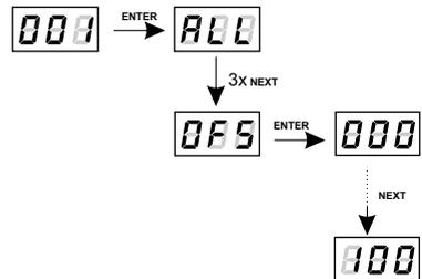
This parameter is useful when the diodes connected to the driver show unstable functioning at the low control levels. In such a case the increase in the value OFFSET can result in achieving better dimming effects.
