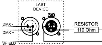
1. To connect the devices application of the microphone cable is strictly recommended (two strands in a shield).
