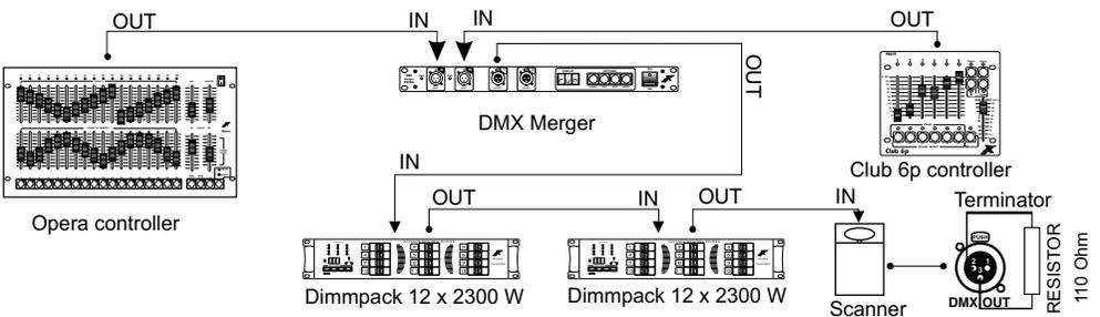
Apart from two-lines summing, the Merger popularises the wide range of possibilities of defining the dependences between inputs. For the precise description see the further part of the manual.
